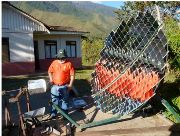
Figure 2: Scheffler concentrator in the test field in Huyro, region of Cusco, Perú
